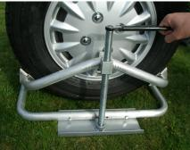
4. Use ratchet to adjust the leveller to desired height.
