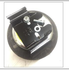
Fasten the Air Spring to the Lower Bracket. Use the M10x1.5-20mm Hex bolts and washers provided.
